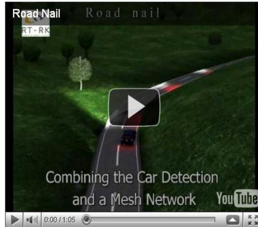
Roadnail product offers road marking based on sensors, wireless connectivity, energy harvesting and light marker as well as local intelligence. It is used to make visible the edge of the road in the front view of a moving car. The system does not need any equipment in the car and therefore works with current car fleet. It is powered autonomously by solar cell on the top of each devices (<http://www.rt-rk.com/new/roadnail>).
